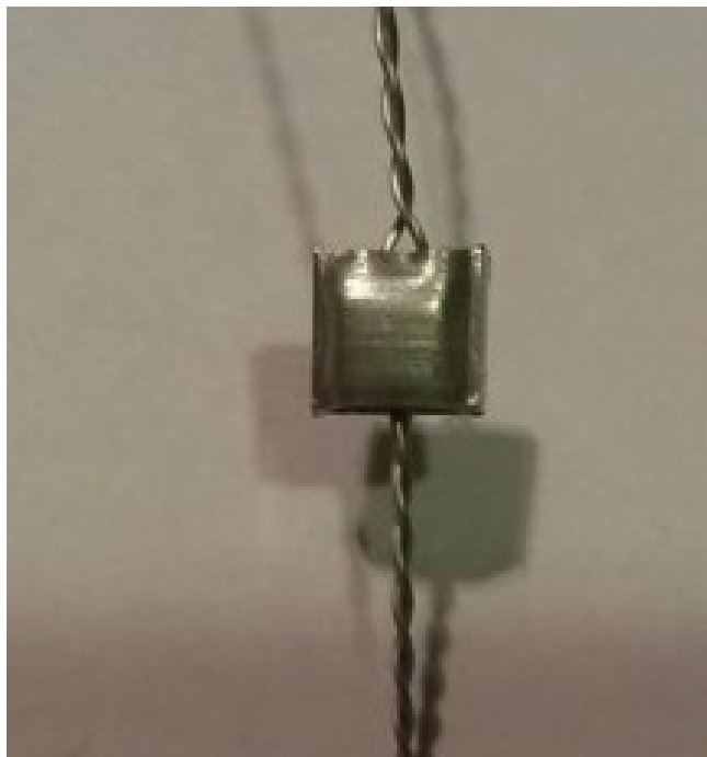
Wire in from side with two holes and out from side with one hole (wire to be wrapped over inside the ALU seal)
