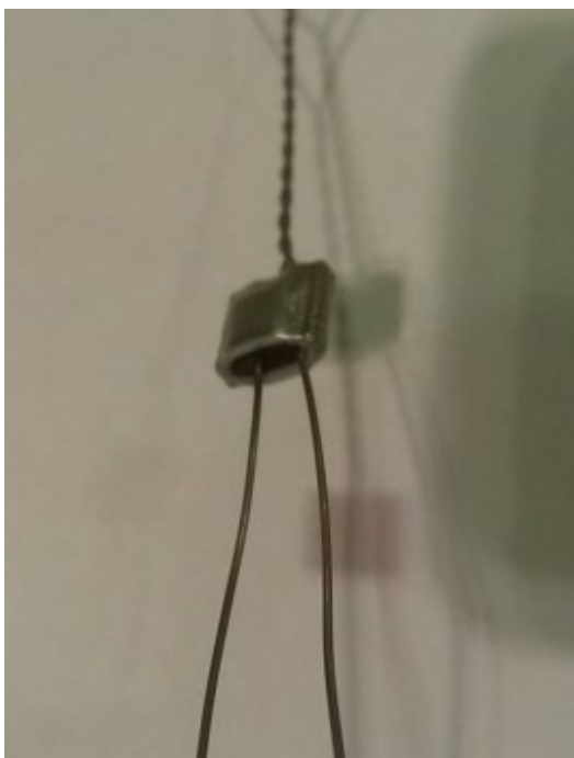
Wire in from side with two holes and out from side with one hole (wire to be wrapped over inside the ALU seal)
